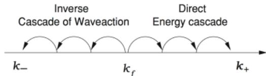
Standard (Fjortoft'1953) argument in 2D turbulence predicts a dual cascade behaviour: energy cascades to low wavenumbers while enstrophy cascades to high wavenumbers. Similar argument in WT predicts a forward cascade of energy and an inverse cascade of waveaction (particles in the GP model).
